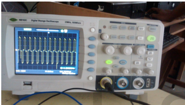
Fig.16: Output Waveform of three level cascaded Inverter
